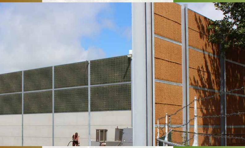
The Kokowall<sup>®</sup> HA-MinWol Noise Barrier is a noise barrier which is finished with natural and durable cocofibres on the outside (covered with climbing plants). On the noiseside the panel has a layer of mineral wool covered with a layer of PE seperator mesh and a galvanised wire netting (without climbing plants).
